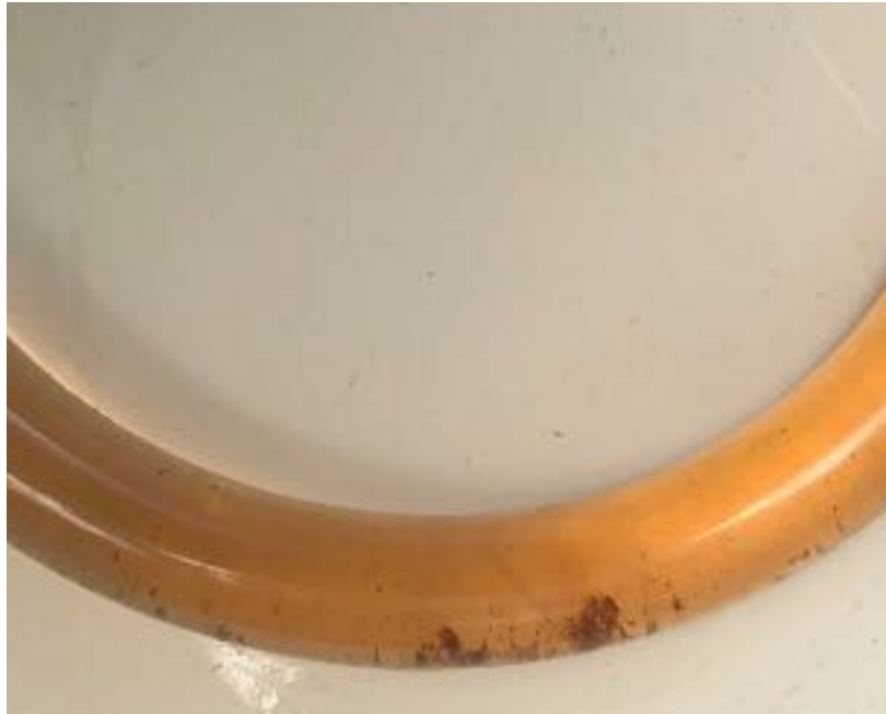
Figure 10: Brown debris in sample taken from fuel tank
