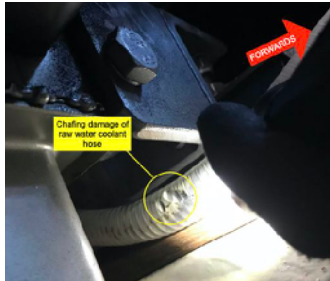
Figure 7: Chafing damage of engine cooling intake hose
