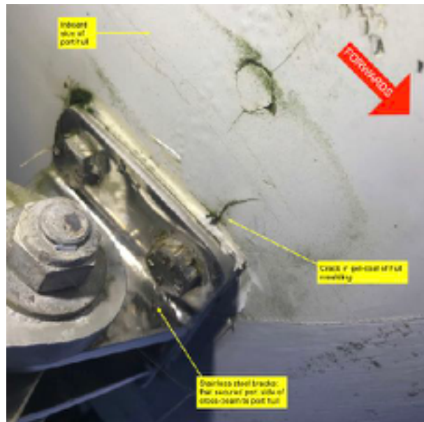
Figure 3: Crack on port hull, where aluminium cross-beam is mounted to hull
