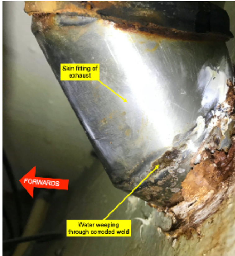
Figure 6: Corroded skin fitting of engine exhaust
