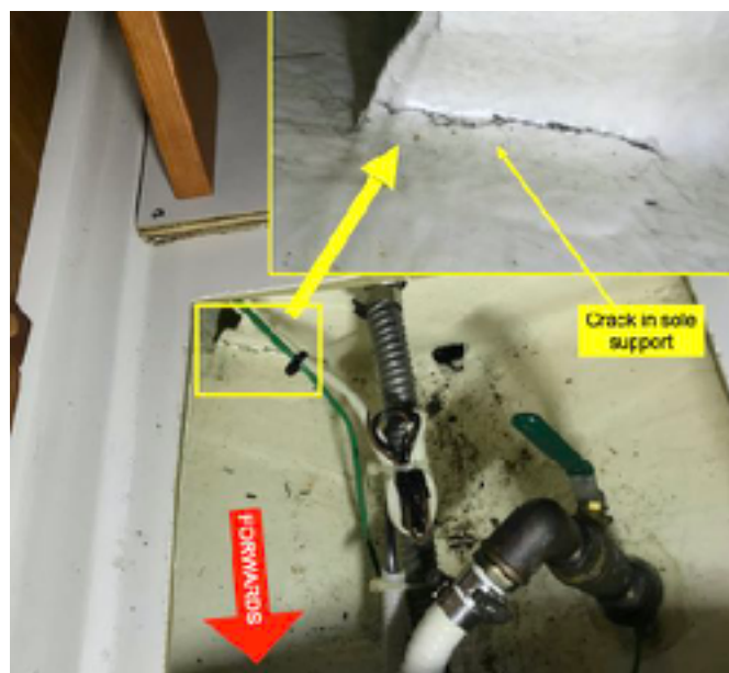
Figure 7: Crack in GRP support of sole in forward living area
