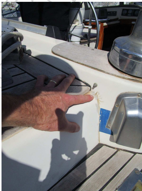
Figure 9: Stress cracks in deck moulding
