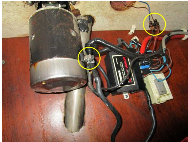
Figure 16: Corroded terminals of anchor windlass
