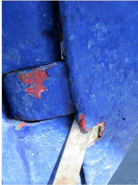
Figure 4: Loose filler next to lower bearing of rudder
