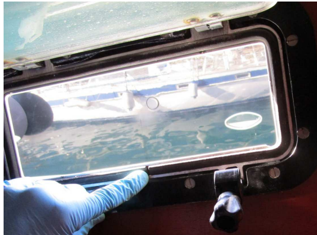
Figure 11: Gap in seal of opening port, forward heads compartment
