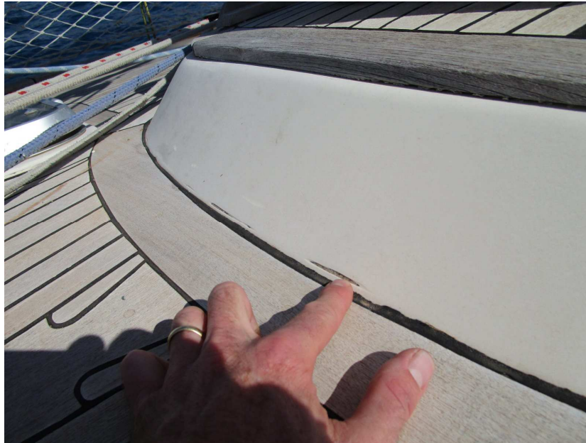
Figure 10: Abrasion damage to gel-coat
