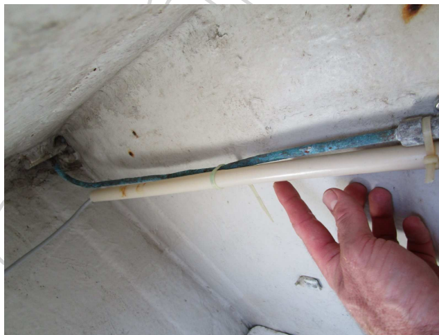
Figure 17: LPG supply pipe in anchor locker
