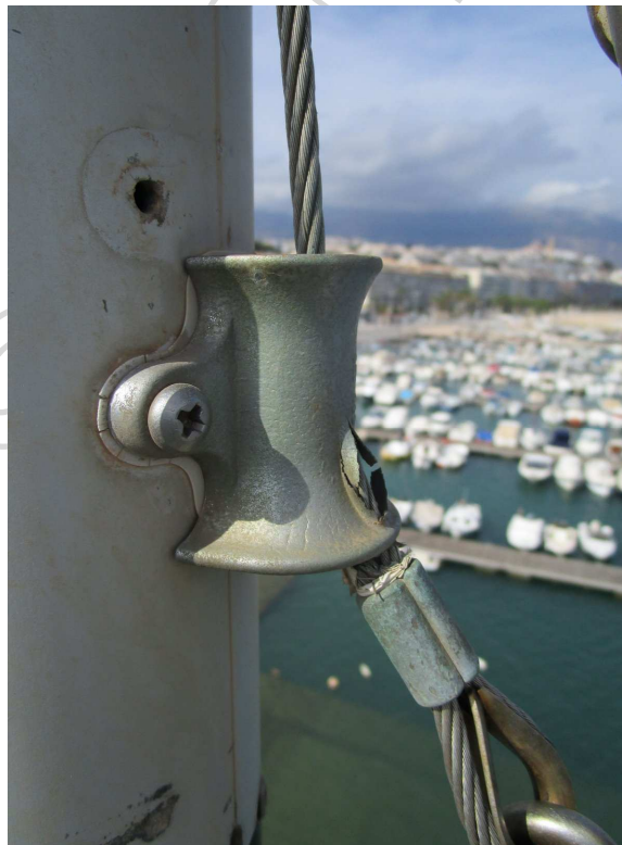
Figure 13: Worn-out sheave at mast head
