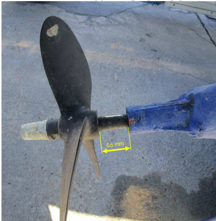
Figure 15: Excessive overhang in propeller shaft
