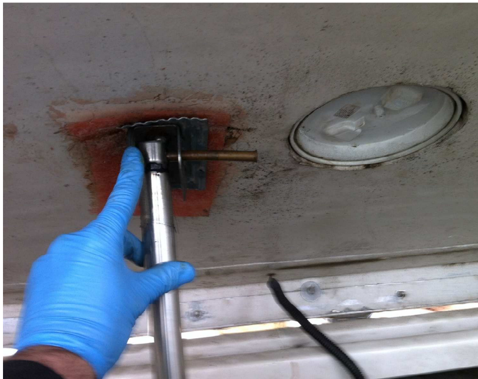
Figure 3: Damage to cockpit sole from engine access lifting strut.
