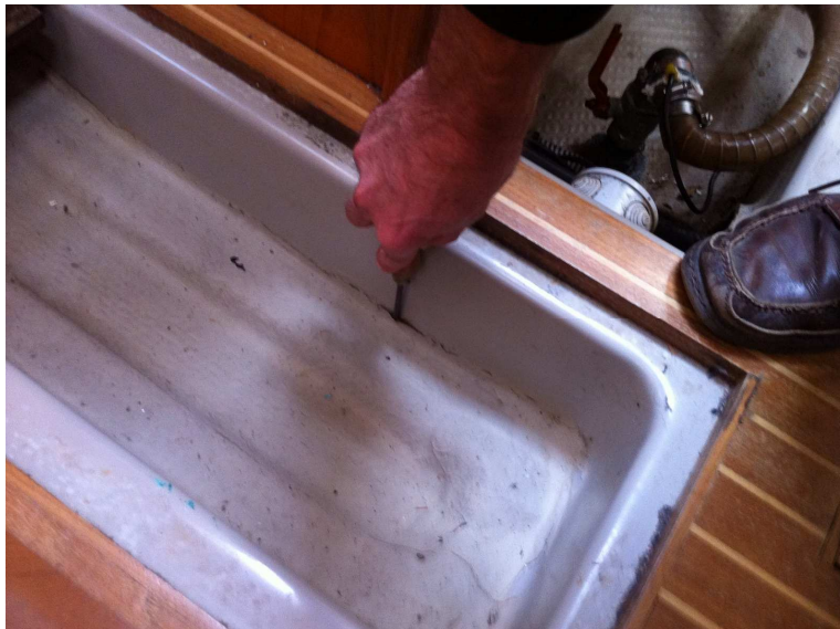
Figure 8: Debonding of tabbing to Internal Moulding laminate
