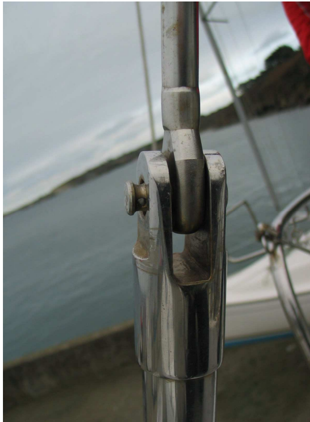
Figure 15: Missing split pin in backstay
