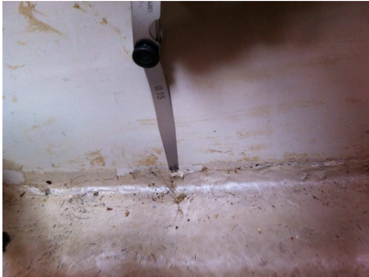
Figure 7: Debonding of tabbing to Internal Moulding laminate
