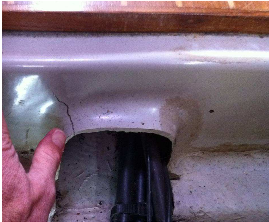
Figure 10: Crack in transverse floor
