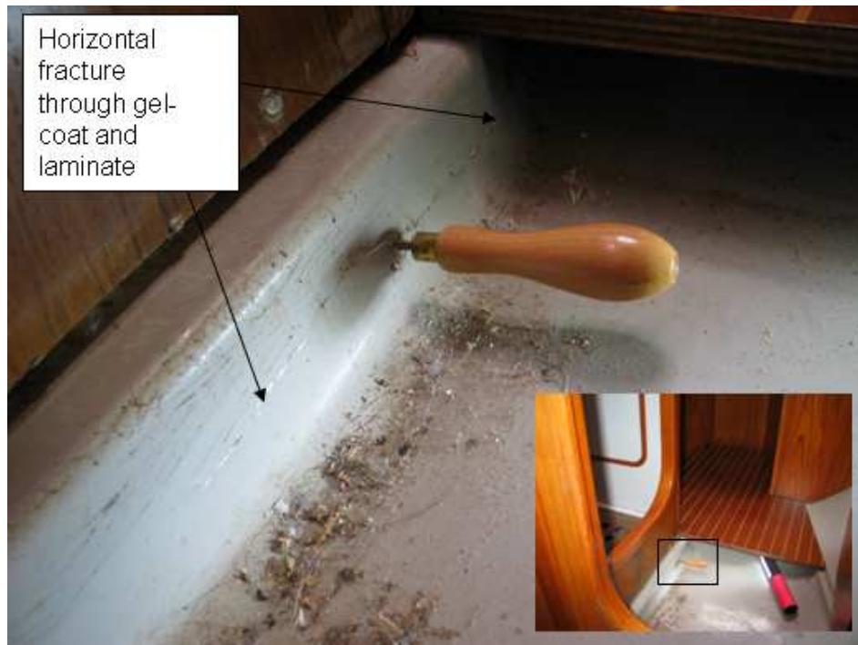
Figure 12: Fracture of Internal Moulding in forepeak
