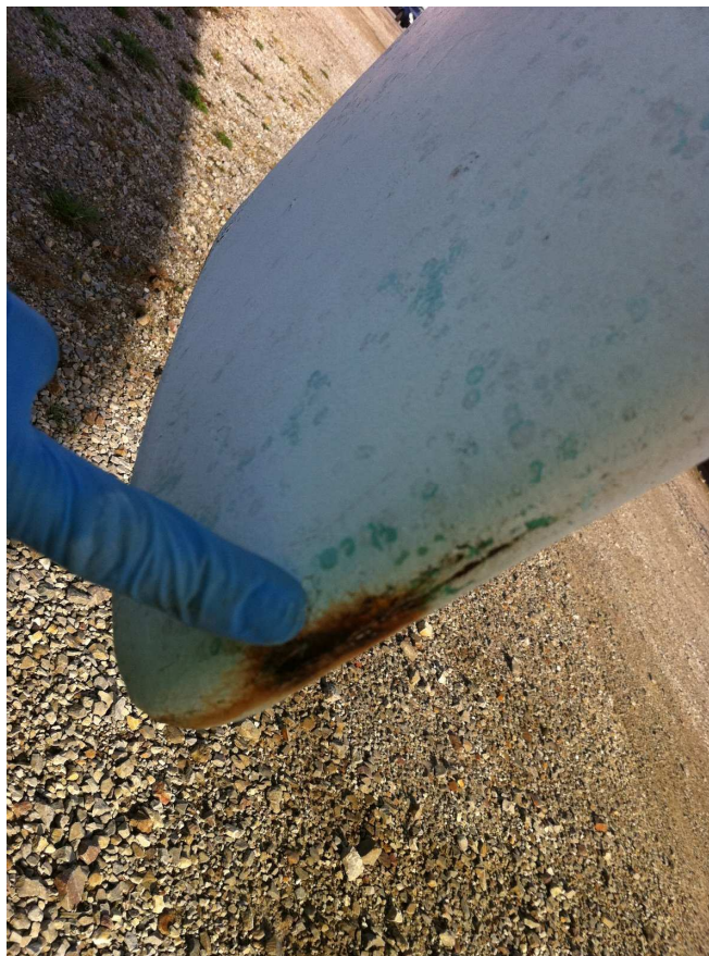
Figure 4: Weeping from crack in leading edge of rudder
