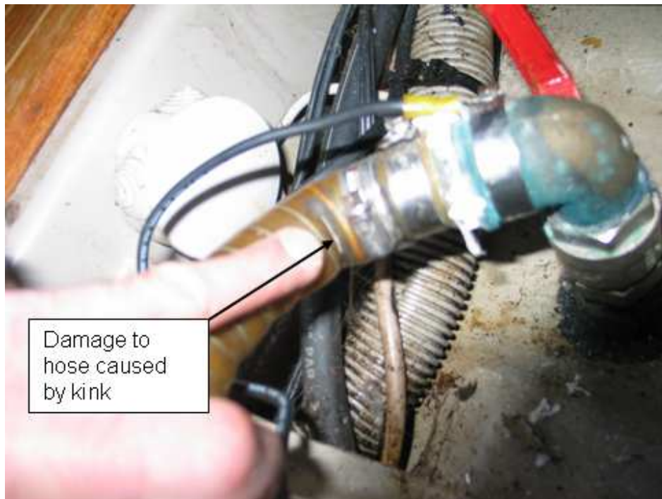
Figure 6: Damage to engine cooling supply hose
